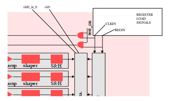
This explains the comment later in the VA1TA manual about the test register only being loaded when the test\_on bit is set.
