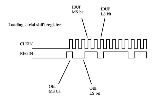
Bit 0 in the bit stream is OBI Most Significant bit.
