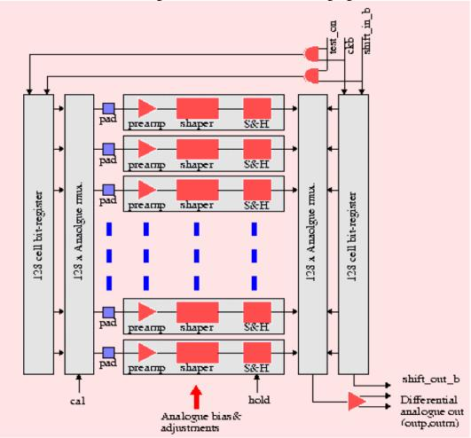
The labels ckb and shift\_in\_b should be CLKIN (Register clock) and REGIN (Register data). The ckb and shift\_in\_b lines should go to the 128xAnalogue mux block in the diagram.
