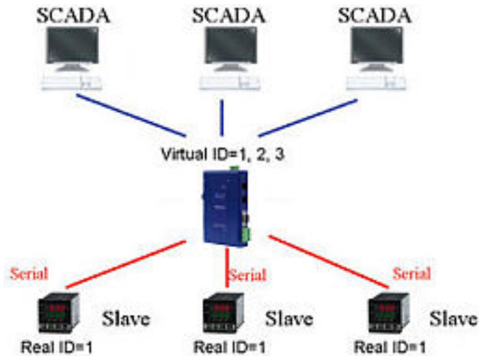
Figure 25. Scada to Slaves, IDs Fixed
