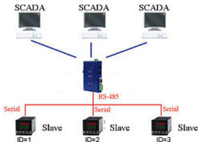
Figure 24. SCADA to Slaves, IDs Configurable
