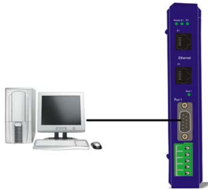
Figure 18. Console Mode Setup
